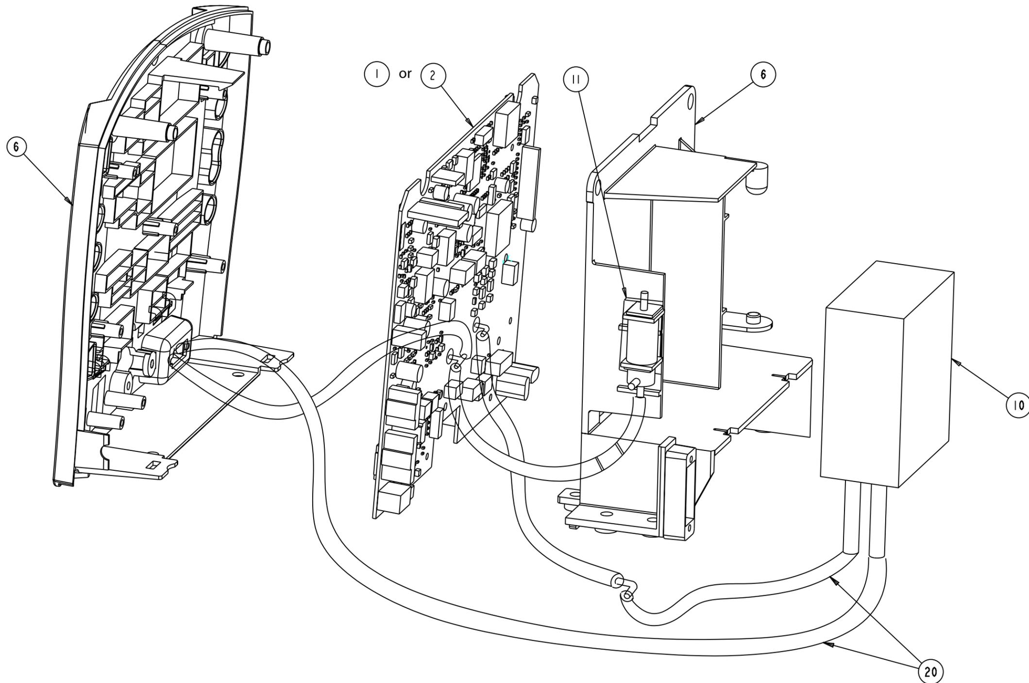
**PNEUMATIC TUBING ROUTING**
