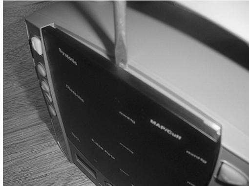
3. Twist the screwdriver so that the display cover is slightly separated from the body of the monitor.
